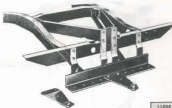
FIG. 330—DRAW BAR MOUNTING
